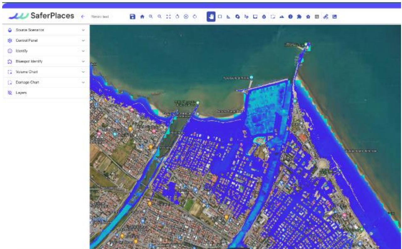
Figure 4: Coastal Flooding with Mean Sea Level at 1.85 m without protection (sandbags) at critical points on the canal port.
